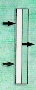
In the same way that this page is inserted into the brochure, the Airfilope® media is sandwiched between two flexible frames. This innovative envelope design allows just the medium to be replaced during routine maintenance, costing less money and creating less waste. This feature allows for a replacement cost that is a mere fraction of the original purchase price.
